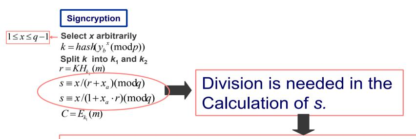
The inclusion of division algorithm in the smart card or mobile terminal increases the size as well as processing time.
