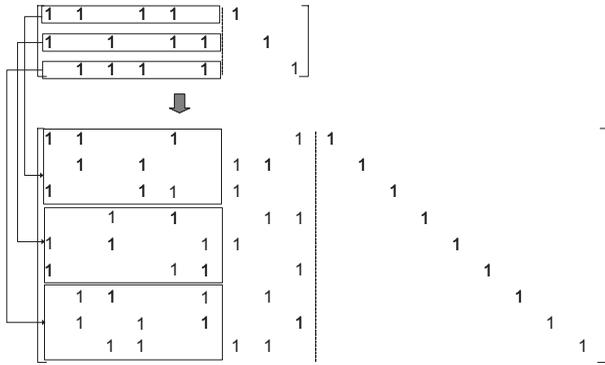
Fig. 2. An (18, 9, 4) inner LDGM code obtained by expanding the rows of the parity check matrix of a (9, 3, 2) outer LDGM code.
