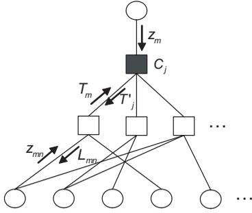
Fig. 4. Modified belief propagation algorithm.
