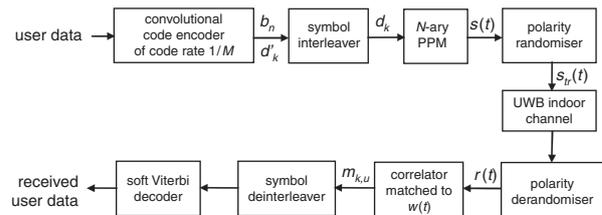
Fig. 1 Coded  $N$ -ary PPM UWB-IR
