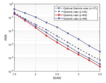
Fig. 2 Performance of the codes using four 6-mark Golomb rulers
