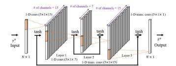
Fig. 2 An illustration of the proposed residual AE denoiser
