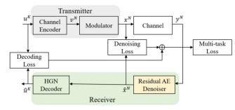
Fig. 1 A system model for the proposed residual AE denoiser
