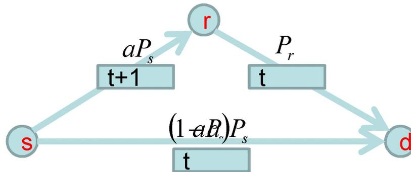
$$R = \max_{0 \leq a \leq 1} \min \left\{ S \left( \frac{\alpha_{sr}^2 a P_s}{N_1} \right), S \left( \frac{\alpha_{sd}^2 P_s + \alpha_{rd}^2 P_r + 2\alpha_{sd}\alpha_{rd}\sqrt{(1-a)P_s P_r}}{N_1 + N_2} \right) \right\}$$
