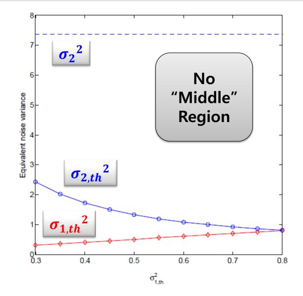
Guideline for the rate allocation for the component codes of Plotkin-type UEP codes.
