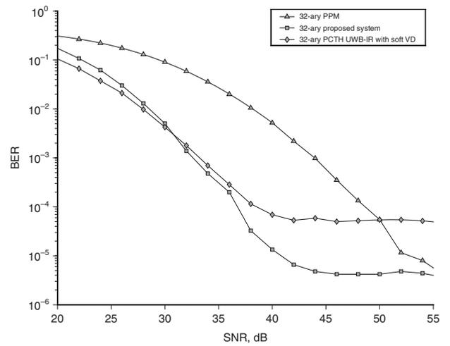
**Fig. 3** BER in UWB-IR indoor channel ( $N = 32$ ,  $T_f = 32$  ns,  $T_s = 1$  ns,  $R_d = 7.58$  Mbit/s,  $T_g = 100$  ns,  $d = 7$  m)
