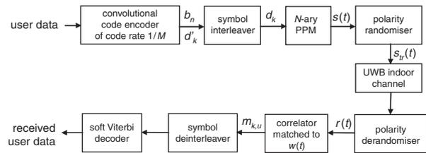
Fig. 1 Coded  $N$ -ary PPM UWB-IR
