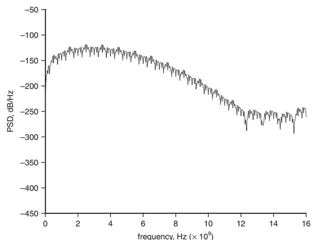
Fig. 2 Actual PSD functions for  $N = 32$ ,  $T_f = 32$  ns,  $T_s = 1$  ns,  $E_s = 1$  W/Hz
