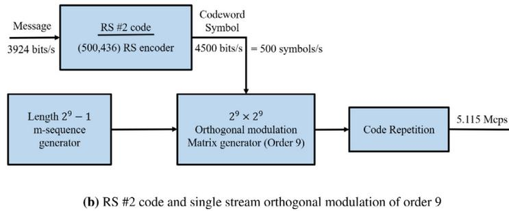
Fig. 2. The proposed RS-coded orthogonal modulation schemes.
