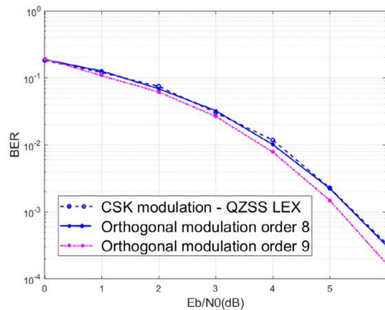
Fig. 3. Performance of three modulation types.
