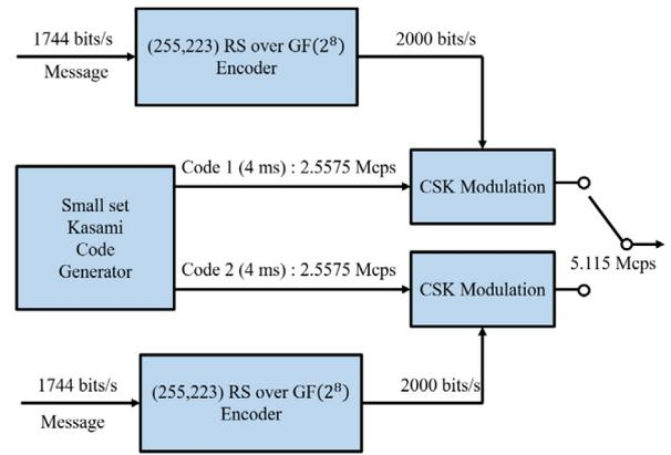
Fig. 1. QZSS-LEX L62 signal structure.
