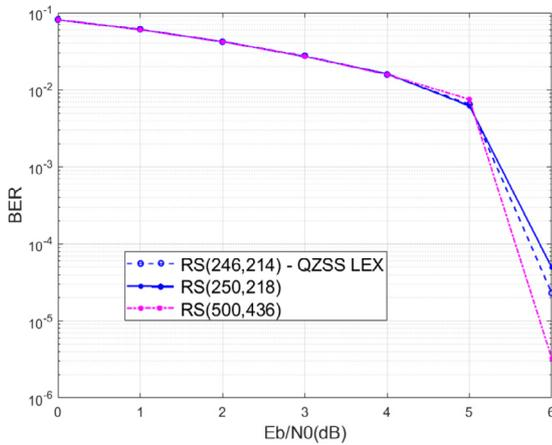
Fig. 4. Performance of three RS codes.
